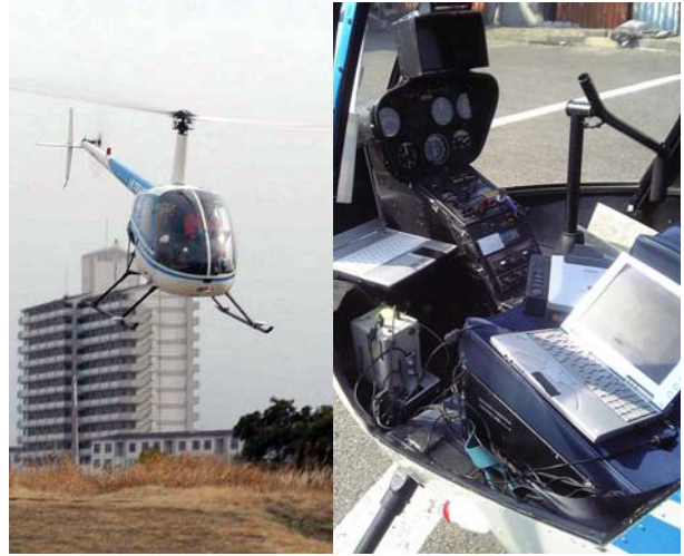
Figure 1 R22 Helicopter and system components for monitoring Urban Heat Island Phenomenon
